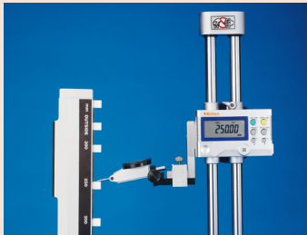
Checking accuracy of height gage
