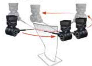
Airfoil section scan
