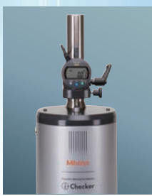
Inspection using digimatic indicator
